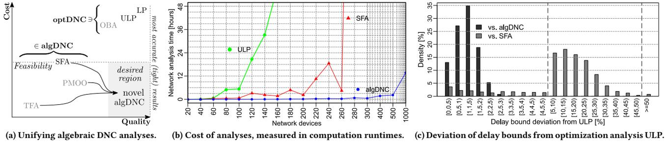
**Figure 1: Evaluation of quality and cost of deterministic network calculus analyses. Among algebraic (algDNC) and optimization (optDNC) analyses, only our novel algDNC achieves the desired tradeoff (a). For the networks feasible to analyze with optDNC’s ULP analysis (b), our delay bounds only deviate by 1.142% on average; a decisive improvement over previous SFA (c).**
