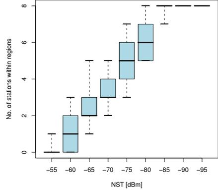
**Figure 2: Box-plot (showing median, lower and upper quartiles, smallest and largest observation) of region sizes for various NST values within our testbed.**
